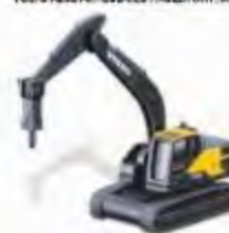
VOLVO EC220B EXCAVATOR WITH REARER
